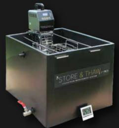
Is an insulated tank with a lid. It has a thermostatically controlled heater and agitator designed to thaw and warm colostrum without damaging the delicate immunoglobulins. It can thaw up to 16 L per hour.
