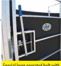
Special lever operated bolt with noise reducing rubber buffers.
