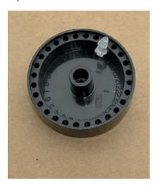
Replace the peg 1 sections to the right, then push the knob back on the spindle taking care to line up the flat face on the spindle with the flat section on the knob. If that is not hot enough, move the peg again one more segments to the right.
